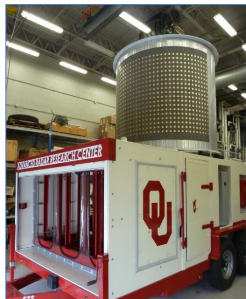
Figure 5: Photo of OU/ARRC Cylindrical Polarized Phased Array Radar (CPPAR) during assembly.
