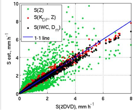
The polarimetric estimates of snow rate are much less sensitive to the variability of snow size distribution than the conventional  $S(Z)$  estimates
